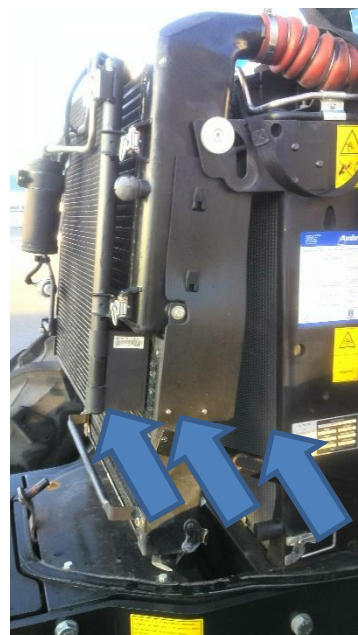
Airco + intercooler + radiator
