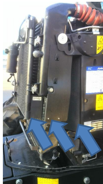
Airco + intercooler + radiator
